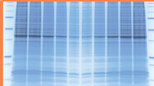
Fig. 2. Results using a stain-free gel are similar to those using a Coomassie-stained gel. Criterion TGX Any kD Stain-Free precast gel run at 200 V for 45 min. Stain-free technology is visualized on the ChemiDoc MP imaging system and compared with a gel stained overnight with Bio-Safe™ Coomassie stain.
